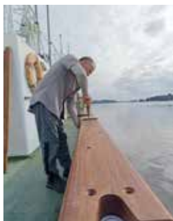
Working vessel replacement Caprail, CMC Design.
